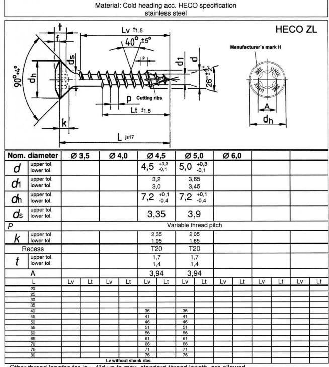
Other thread lengths for  $lg \ge 4^*d$  up to max. standard thread length, are allowed
