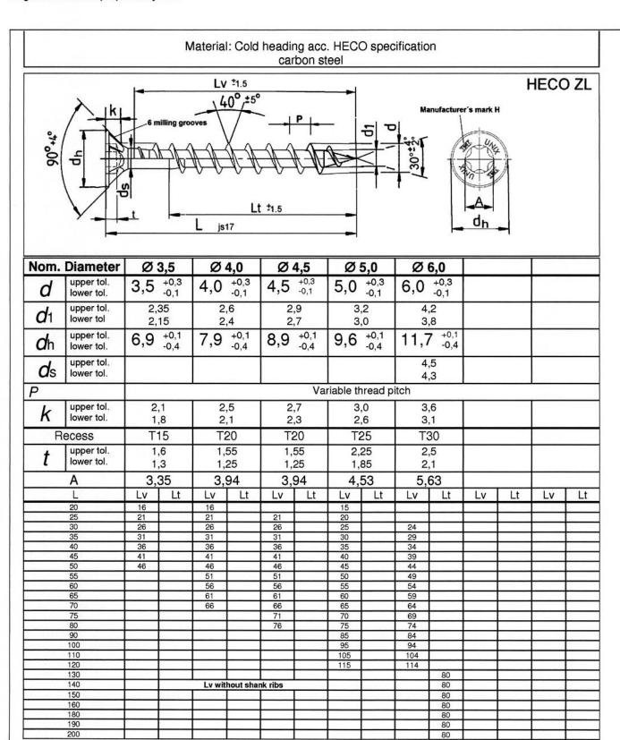
Other thread lengths for  $lg \ge 4^*d$  up to max. standard thread length, are allowed
